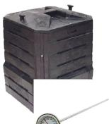
The **Rapitest Compost Thermometer** has a large, easily-read dial and a 19" stainless steel probe with a range of 0-220 degrees Fahrenheit, so growers can accurately measure the internal temperature of their pile.
